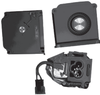
Fans and AC power inlet
