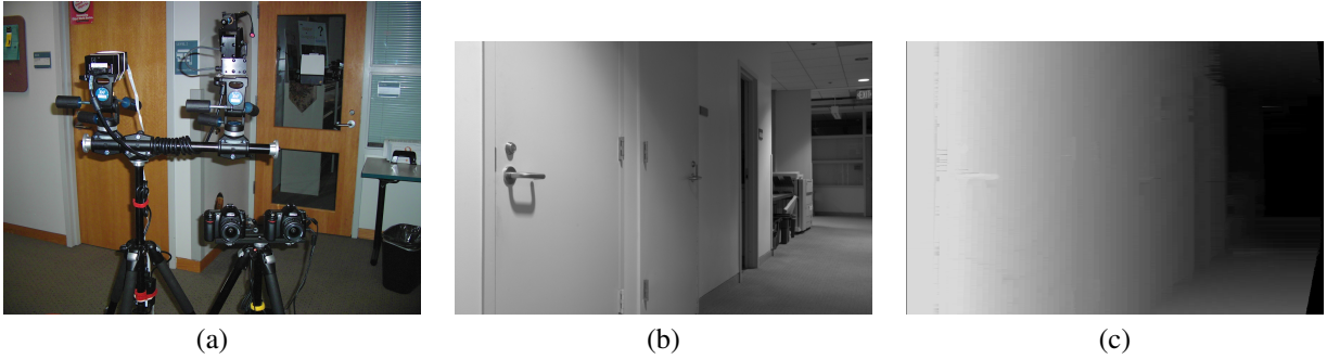
Figure 12: (a) Our prototype camera/laser apparatus, (b) Our hallway, (c) Disparity map after 200 laser aims.
