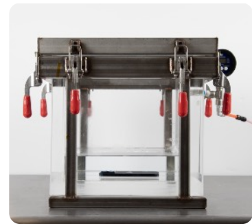
To test for IPX7/8 water immersion protection, Apple submerge iPhone inside a pressurised vessel to simulate pressure experienced underwater.
