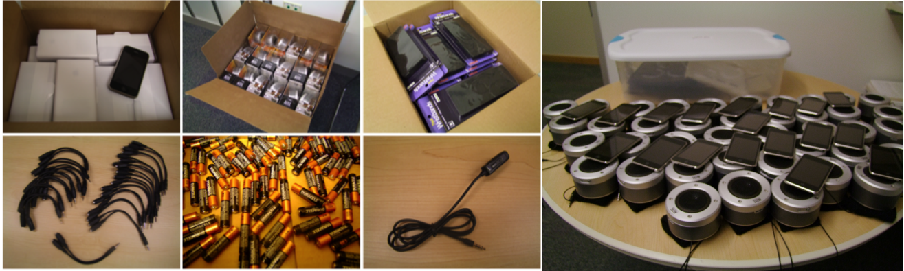
Figure 1. Equipment needed to set up the ensemble: iPod Touches, portable speakers, tennis wristbands, y-collectors, lots of batteries, external microphone (left to right, top to bottom). Completed ensemble instruments after sewing the wristbands to the speakers. All equipment can easily be transported in laundry crates (right)
