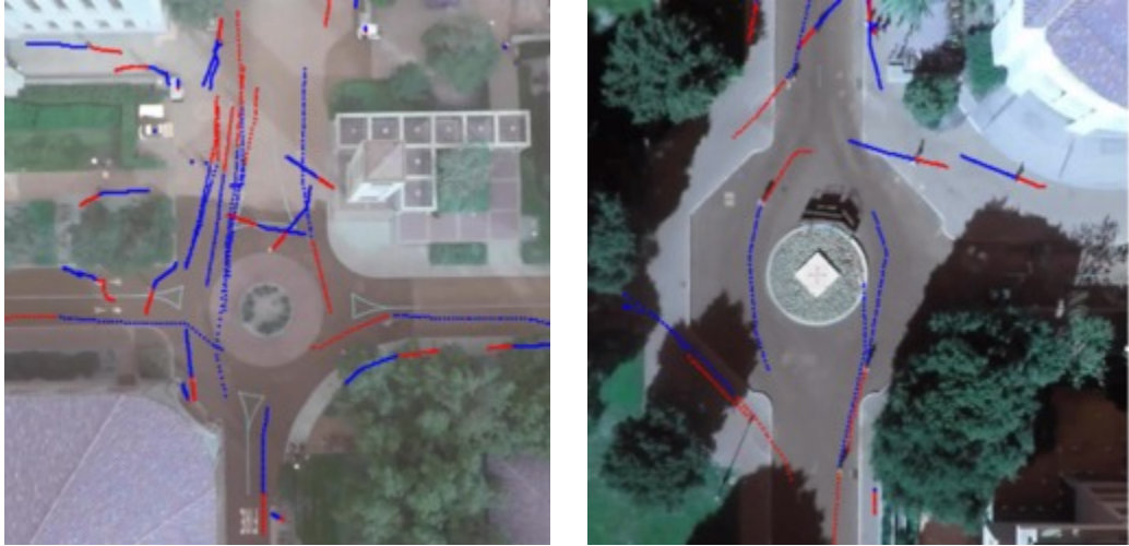
Figure 1.1: Example of real traffic scenario of several agents moving in the scene. Taken from [49]. Red and blue depict past and future motions respectively. Agents can be seen to be moving subject to the scene (road, roundabout, side-walks etc) and ensuring no collisions with each other.
