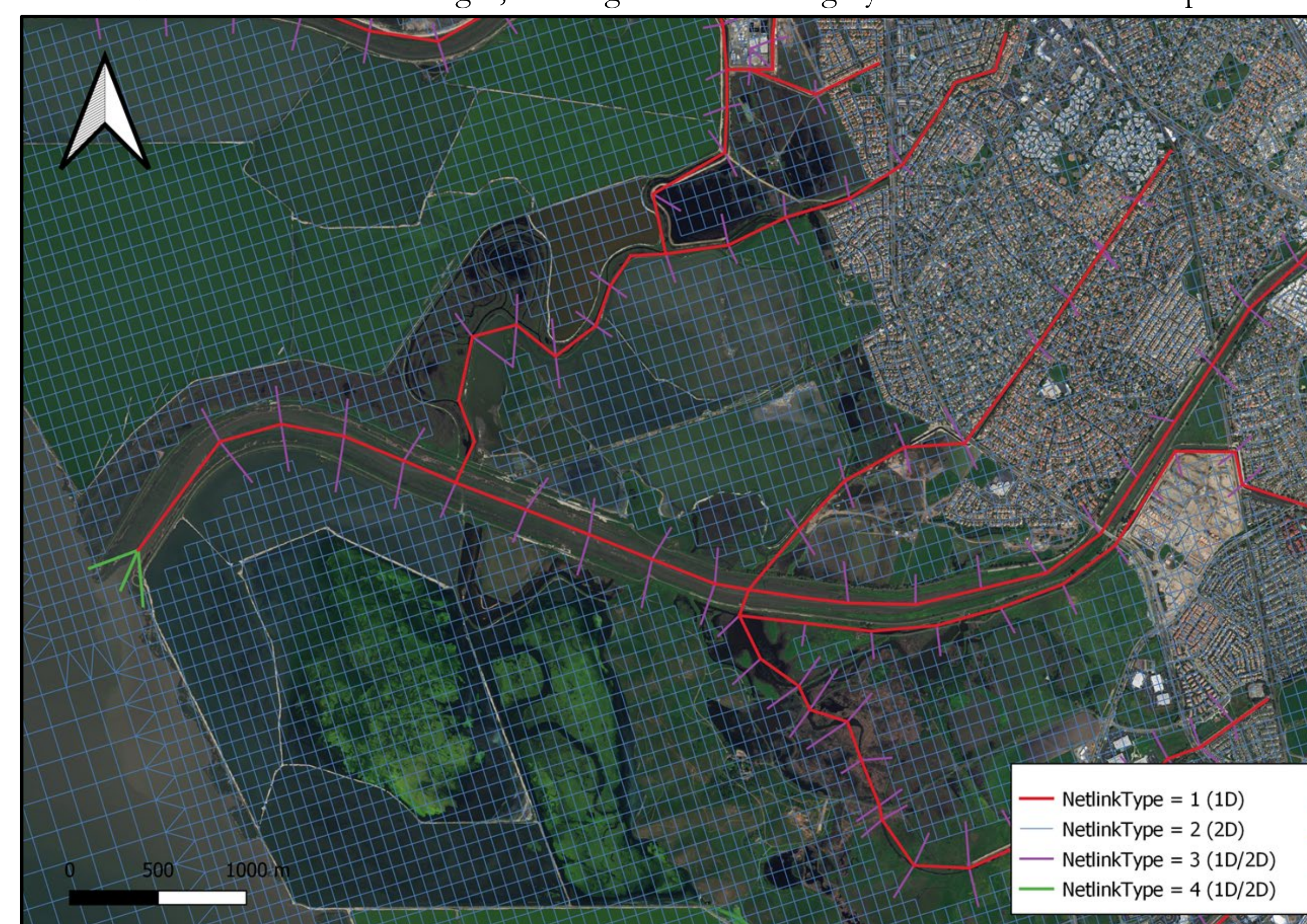
Figure 4 Close up view of how the 1D channels are integrated with the 2D mesh.
