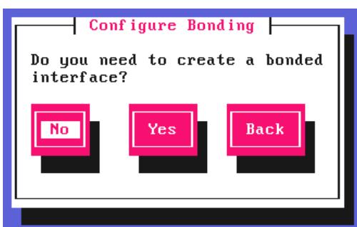
If you select **Yes**, the **Select Interfaces** screen will be displayed. Using the space bar, select the interfaces you'd like to include in the bond, select **Create** and hit <ENTER> to continue.
