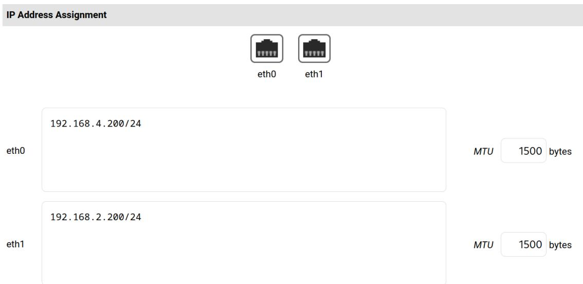
4. Configure the required IP address for **eth0**, e.g. **192.168.4.200/24**.
