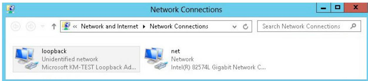
**① Important** Either adjust the commands to use the names allocated to your LAN and loopback adapters, or rename the adapters before running the commands. Names are case sensitive so make sure that the interface names used in the commands match the adapter names exactly.
