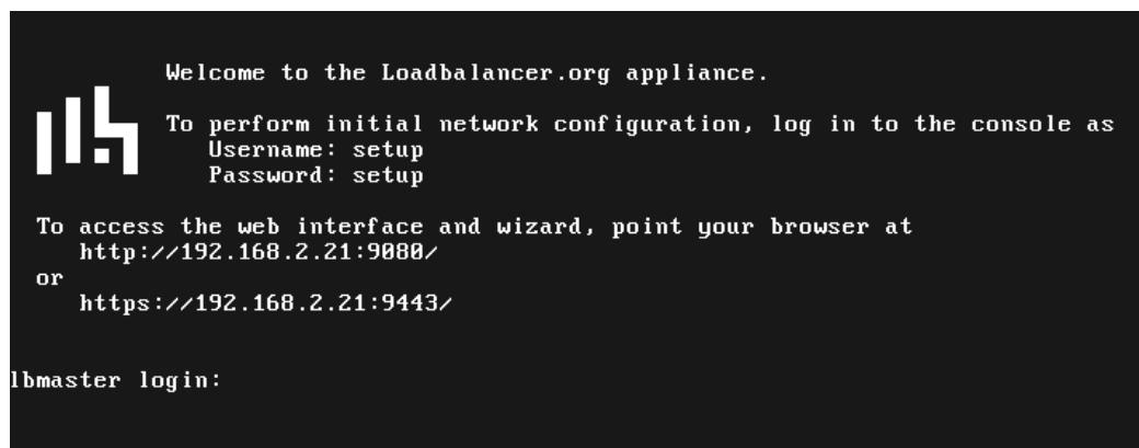
As mentioned in the text, to perform initial network configuration, login as the "setup" user at the appliance console.
