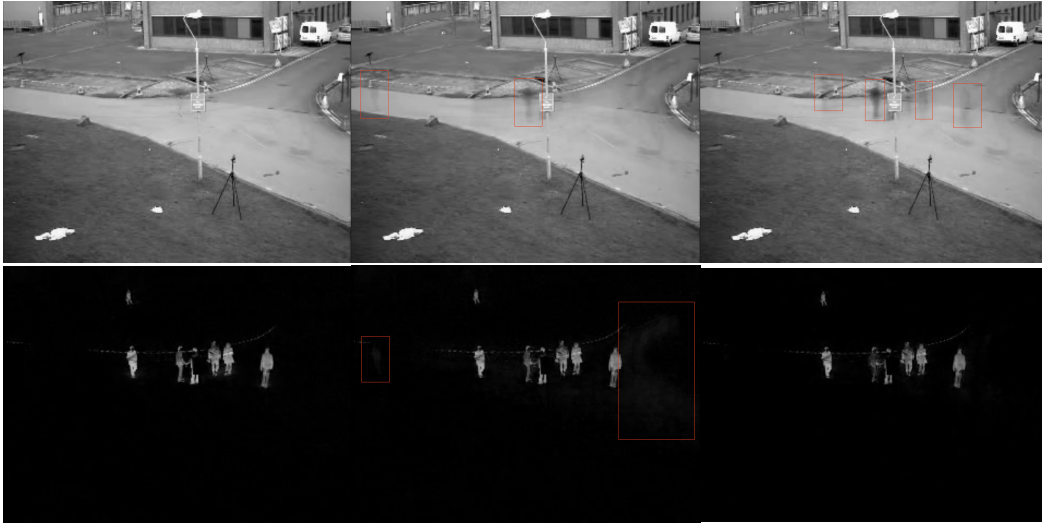
Figure 2: Foreground-background separation from video. From left to right: Fast Greedy with rank=3 and Huber loss with \delta = 20 . Standard PCA with rank=1. Principal Component Pursuit (PCP) with \lambda = 0.002 . Both PCA and PCP have visible "shadows" in the foreground that appear as "smudges" in the background. These are less obvious in a still frame but more apparent in a video.
