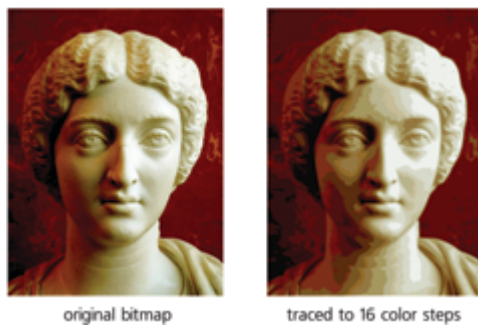
Figure 14: A bitmap image (left) and a group of colored vector paths (right) created by the Trace Bitmap dialog in Multiple scans mode with 12 colors (page 313).
