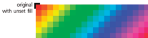
Figure 10: A rainbow pattern created by the Create Tiled Clones dialog, Color tab; you start with a single rectangle with unset color and set the original color as well as the amount of change for each color channel per row and per column (page 283).
