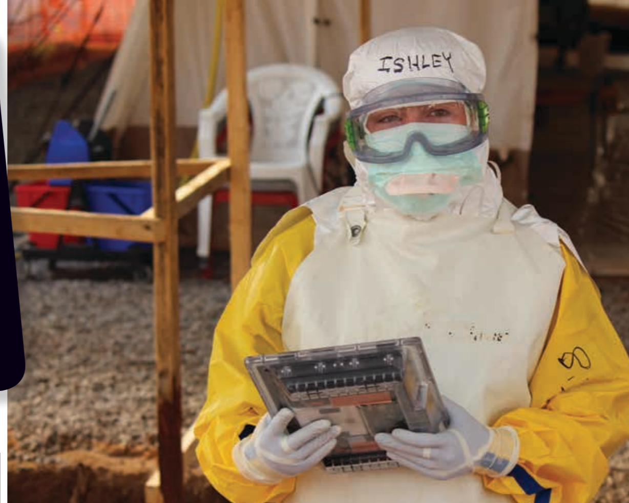
The tablets have no sharp edges, which might puncture protective clothing, and they are simple to use even when wearing three pairs of gloves. Photograph © Nick Fortescue
