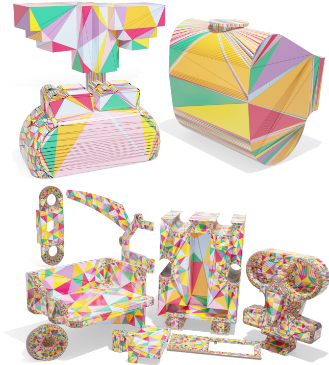
Fig. 12. Using our integer-based data structure, we can not only improve near-degenerate meshes by generating intrinsic Delaunay triangulations (top), but can also extract the common subdivision after computing a high-quality intrinsic Delaunay refinement (bottom).
