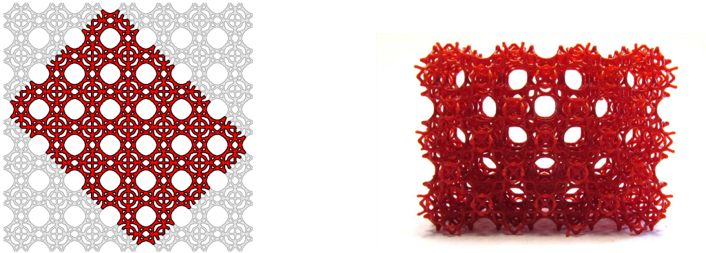
Figure 3.6: We extracted a 45^\circ rotated rectangular block from a regularly tiled 10mm cell microstructure to test Young’s modulus in non-axis aligned directions.
