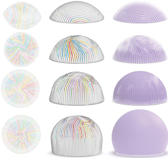
Fig. 12. Not all shapes can be inflated from a single patch. For increasingly larger parts of the sphere, metric distortion eventually exceeds the bounds realizable by the limited air channel contraction, leading to increasingly larger deviations from the target shape.
