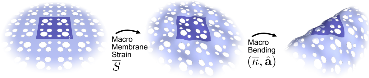
Figure 3 Deformations applied to an infinite periodic sheet tiling during homogenization (left): first an in-plane constant macroscopic stretch is applied and the sheet relaxes into a (potentially non-planar) periodic fluctuation displacement around the linear deformation (middle). Second, the entire tiling is bent into a surface of constant curvature (right).
