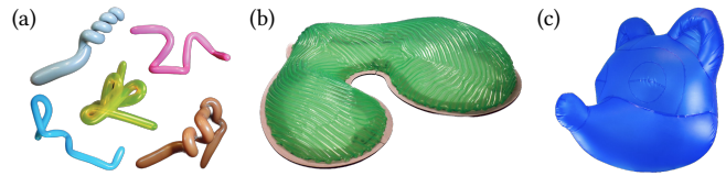
Fig. 3. Representative examples of existing works on inflatables: (a) curve inflatables [Baines et al. 2023], (b) surface-based inflatables [Panetta et al. 2021], and (c) volumetric inflatables [Skouras et al. 2014]. Copyrights for the three images are held by the authors of the cited papers.
