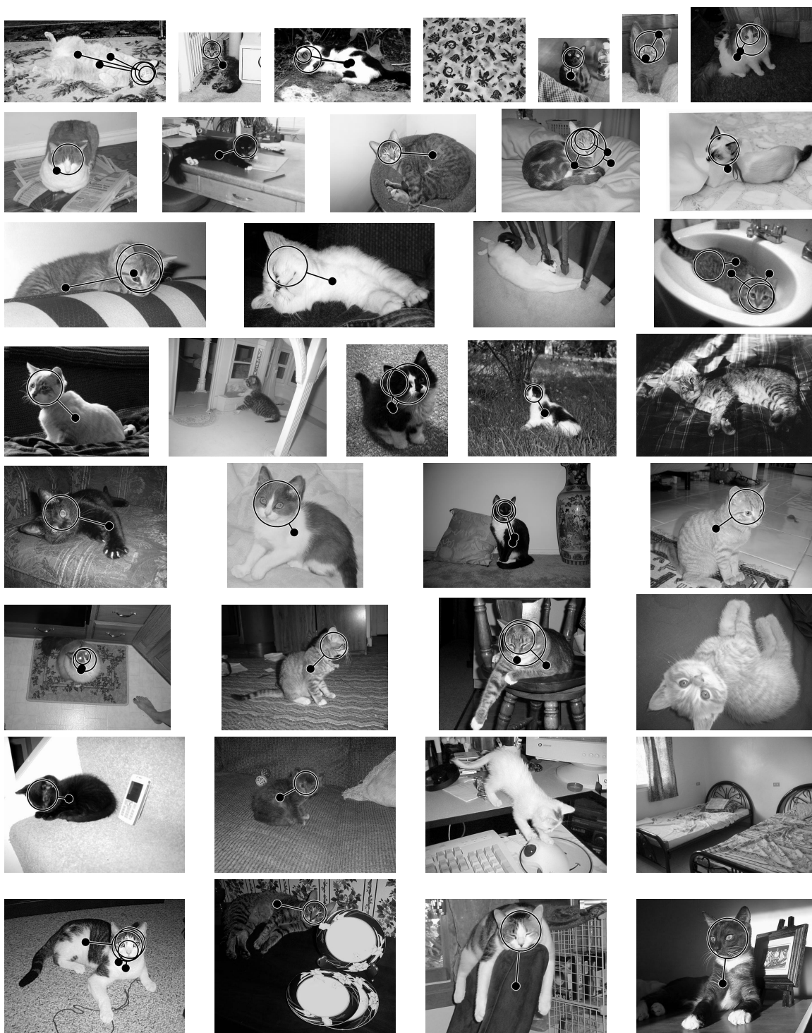
Figure 14: Detection results with stationary features and a folded two-level hierarchy on scenes picked uniformly at random in the RateMykitten test set, with a true-positive rate of 71%. The circle shows the estimated head size and location, and the dot the estimated belly location.
