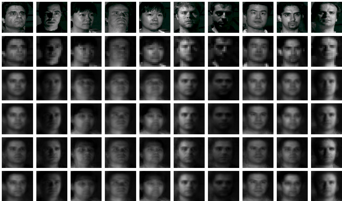
Figure 9: Rows from top to bottom: Original face images ( 60 \times 60 pixels); sub-sampled images ( 20 \times 20 pixels); super-resolution images produced by KHA after one pass through the data set; likewise for KHA-SMD.
