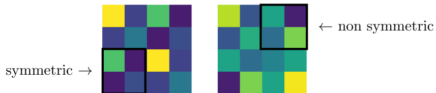
Figure 3: Illustration on differences of separable (left) and non-separable (right) operator-valued kernels. For separable kernels the p \times p output matrix is always a psd symmetric matrix.
