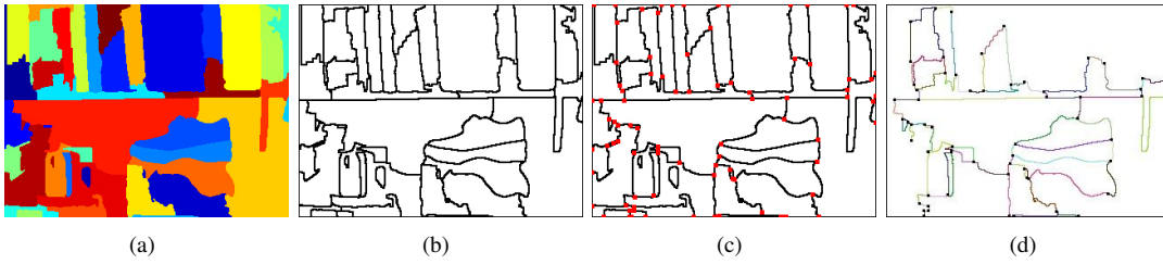
Fig. 3. Generating a graph from an over-segmented image. (a) an over-segmented image (b) an edge map extracted from the over-segmented image (c) extracted nodes (red rectangles) (d) final graph (the edges passing the image boundary are omitted).
