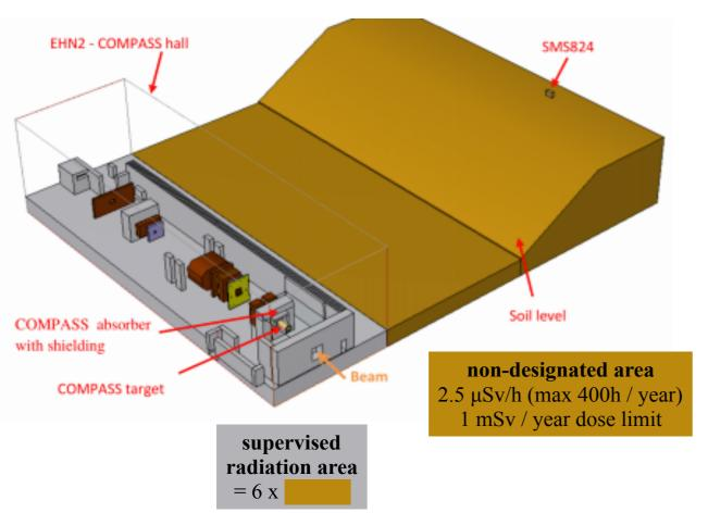
• FLUKA simulation of COMPASS 2018 run.
