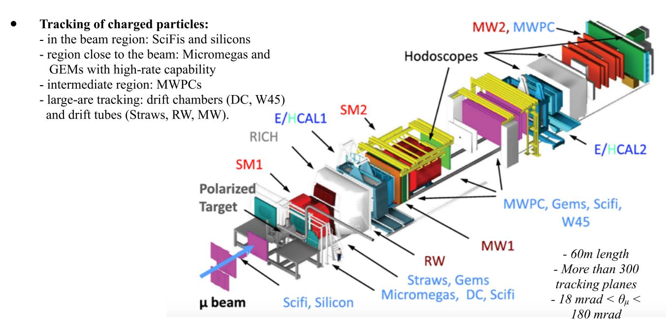
Separation of produced pions & kaons: RICH with multianode-photomultiplier tubes and MWPCs with photosensitive CsI cathodes in the periphery
