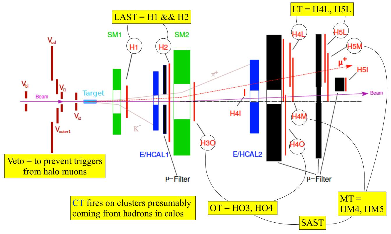
OT, MT, LAST = target-pointing triggers LT, IT = energy-loss triggers
