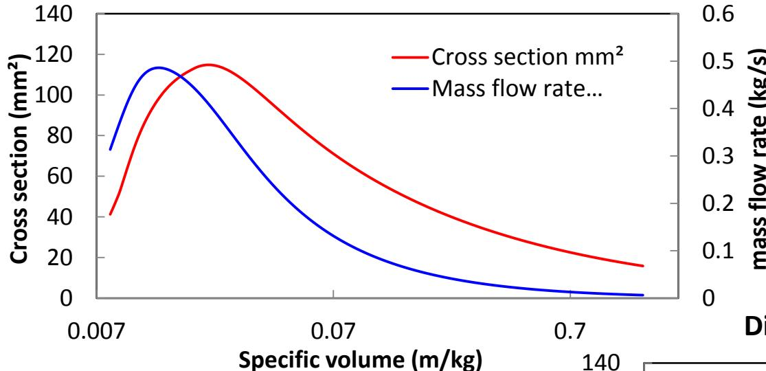
Maximum mass flow rate and cross section not for the same specific volume
