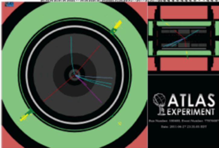
Event display of highest mass di-electron event from ATLAS Z' \rightarrow ee search
