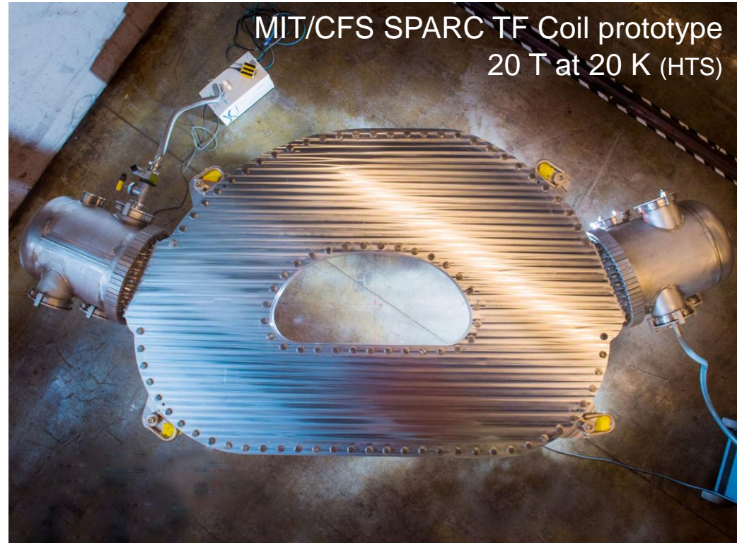
Compact fusion reactors, based on HTS
