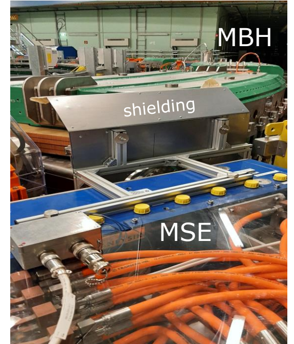
One of the countermeasures tested: shielding the MSE dipole from the MBH dipole.
