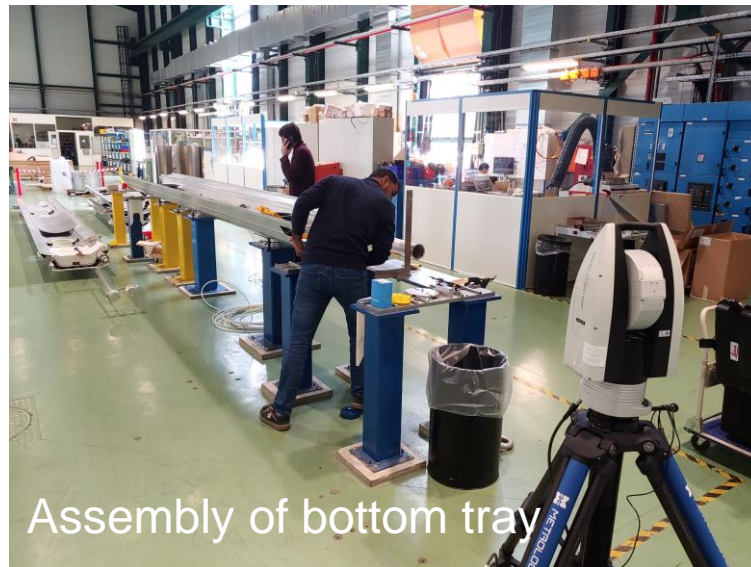
Alignment of coldbore tubes
