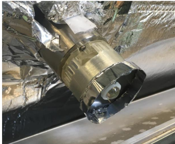
Reflecting target (glass sphere) on cold mass
