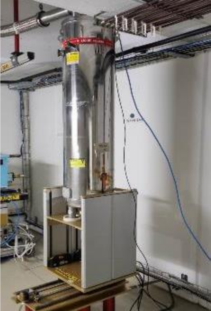
He cryostat for proton irradiation at IRRAD facility with support of the Cryolab (CERN),
