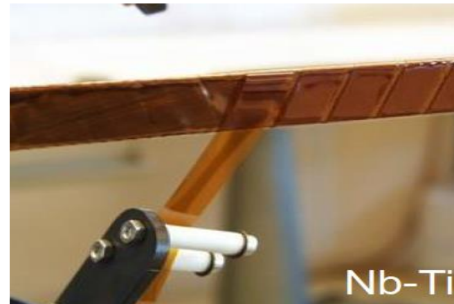
Fig. 2. Layout of cable insulation of the LHC main dipoles and quadrupoles. The detail of the 3rd layer is shown, which consists in a 9 mm wide tape, wrapped spaced by 2 mm to allow helium to penetrate in the coil, adhesive on its outer side to bond adjacent coil turns together.
