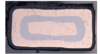
Nb-Ti PVA insulated. Ribbon cable made of 15 Nb-Ti wires and impregnated with epoxy (MCBY corrector)
