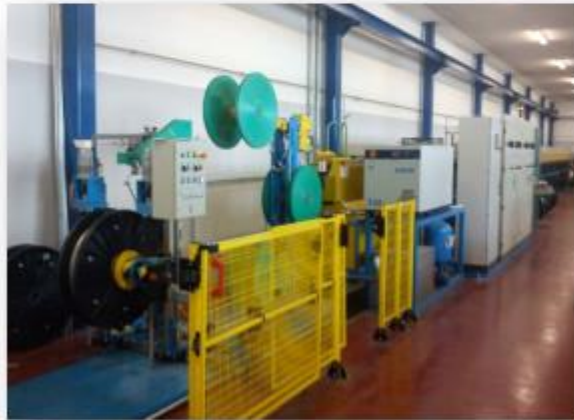
20 m long in-line furnace
