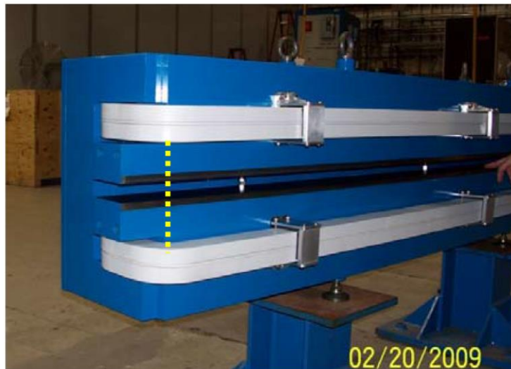
Figure 1: Prototype magnet for NSLS-II with “ extended pole ” or “ nose ”. The dotted line shows the boundary between the nose piece and the main laminations.
