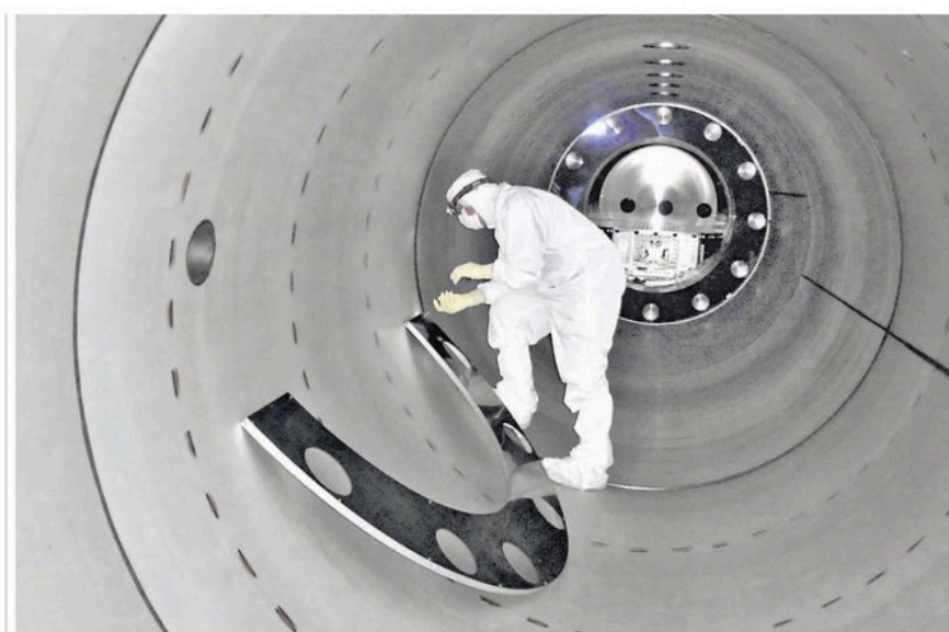
A worker installed a baffle in 2010 to control light in the Laser Interferometer Gravitational-Wave Observatory in Hanford, Wash.
