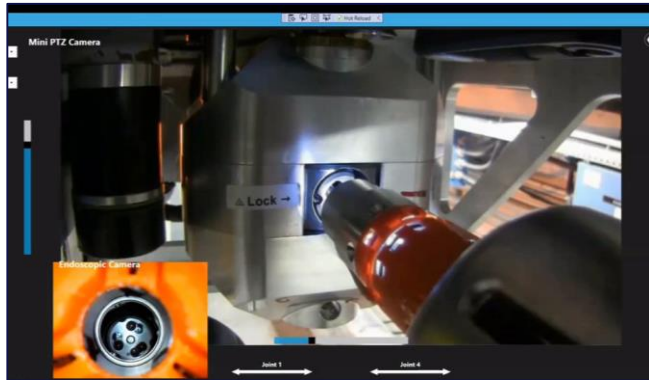
TIM Handling Radioactive Source for BLM Tests
