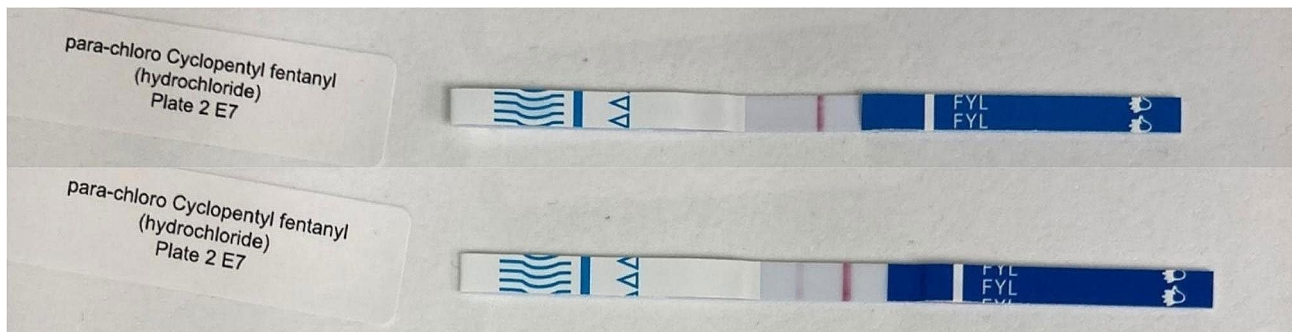
Fig. 3 Lot to lot variability: Top: BTNX lot 2,204,104 gives positive result; Bottom BTNX lot 2,206,394 gives negative result. Para -chloro Cyclopentyl fentanyl at 20,000 ng/mL
