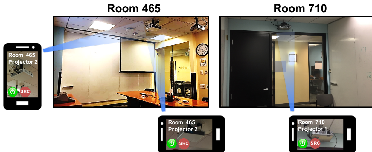
Figure 4.1: Application scenario for our vision-based appliance identification and control system. Users can get a control interface of an appliance by capturing an image from an arbitrary angle and distance, even when other similar appliances exist in the same or different rooms.
