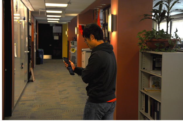
Figure 3.4: Experimenter holds two smartphones while walking in the office space. One smartphone is collecting both WiFi RSSI and ABS fingerprints, and the other one is capturing a video for manual ground truth inference.
