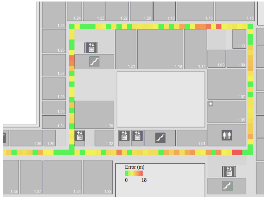
Figure 3.7: Spatial distribution of WiFi fingerprinting based location estimation errors on the floor plan.
