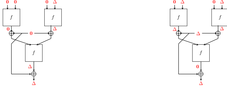
(a) Processing of message m = (\mathbf{0}, \mathbf{0}, \mathbf{0}, \Delta, \mathbf{0}) through T_5^f (b) Processing of message m' = (\mathbf{0}, \Delta, \mathbf{0}, \Delta, \Delta) through T_5^f
