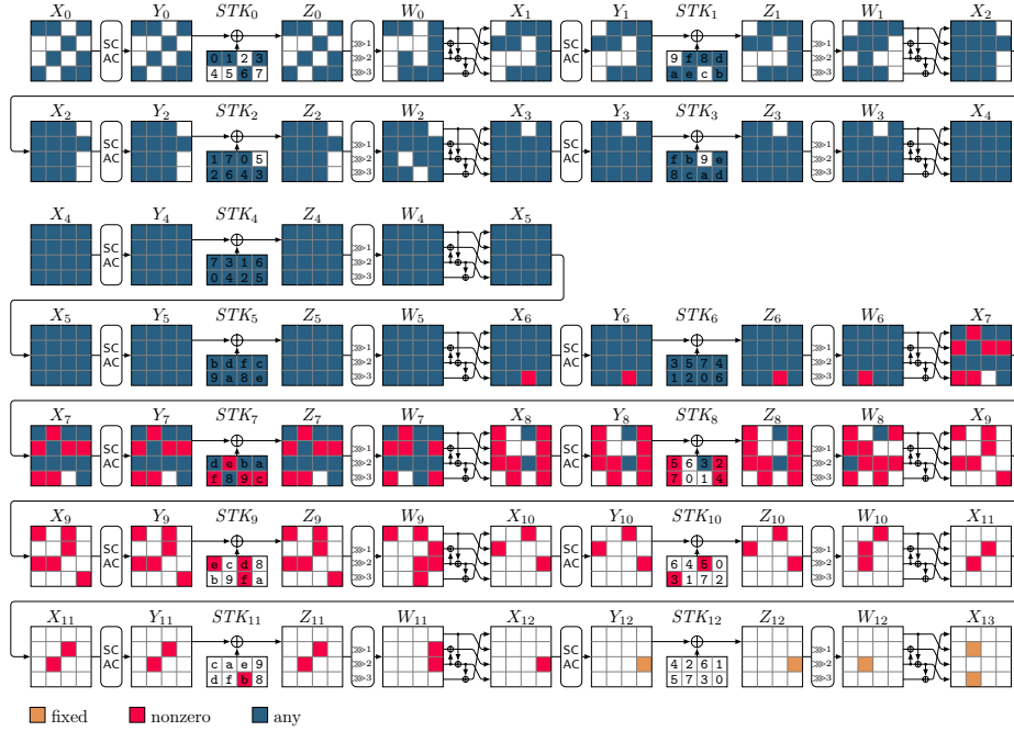
Fig. 24: ZC-Integral distinguisher for 13 rounds of SKINNY- n-2n . STK[9] is active at most two times. X_{13}[5] \oplus X_{13}[13] is balanced. Data complexity: 2^{9 \cdot c} , c \in \{4, 8\} .
