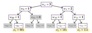
Figure 2: An example prefix tree on strings  $(\alpha_1, \alpha_2, \alpha_3)$  of length n = 3. The weight  $w_p$  of a prefix  $p \in \{0, 1\}^*$  is the number of strings in the tree that have p as a prefix.
