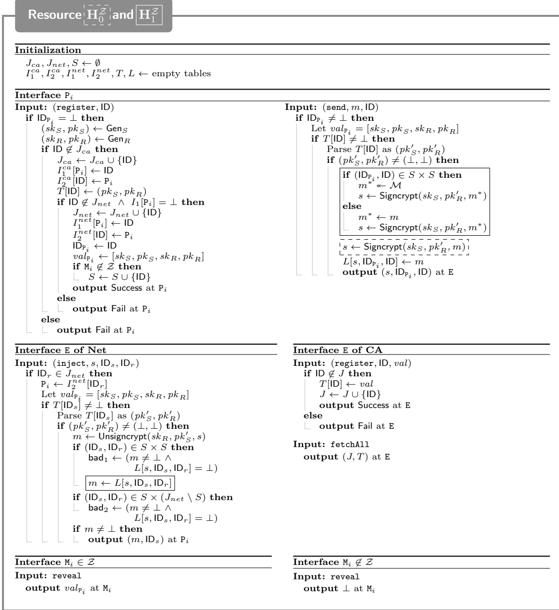
Fig. 16. The second hybrid system replaces encryptions of messages between honest parties by encryptions of uniform random messages. In addition, a message between two honest users is only delivered if it was recorded in L with the matching identities. The difference of these two hybrids can be bounded by the real-or-random game of Signcrypt in the outsider security model.
