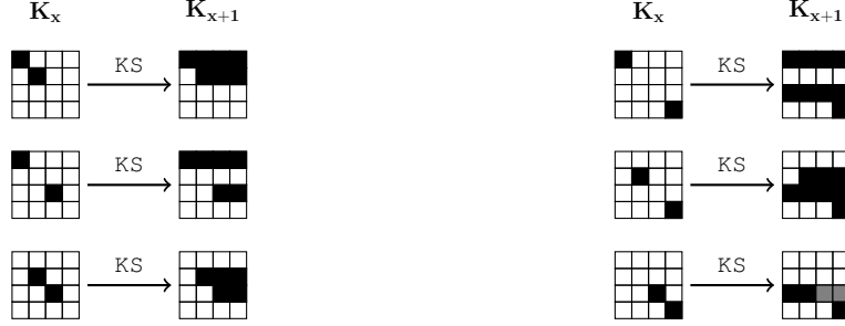
Figure 9: Key schedule patterns for two active bytes located in the same diagonal.
