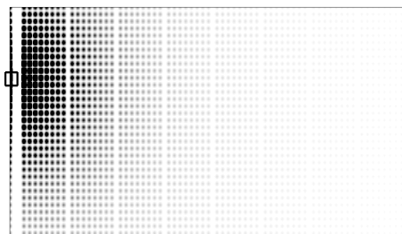
Fig. 5. Simulated photonic emissions received by the detector (in a box) from the various transistors of the simulated SRAM structure over 1ms. The darkness of a point indicates the quantity of photons emitted from that point towards the detector.
