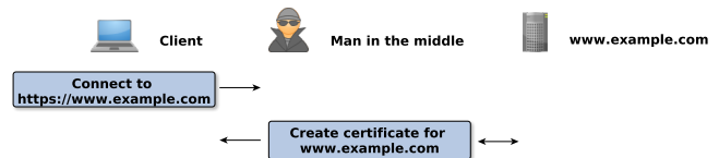
Figure 12: Basic mode of operation of sslsniff - Impersonating a server
