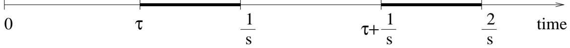
Figure 2-11: A schedule for the I-O pair (i, j) . The pair gets a service opportunity at the end of each frame.
