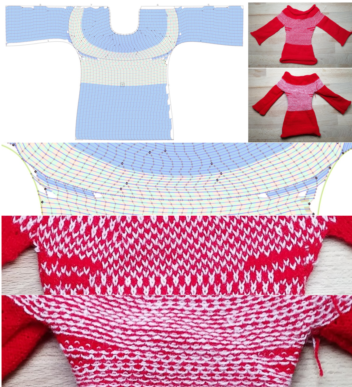
Figure 6-41: Example of simple float pattern that does not require any tuck pattern because the tiled checkerboard pattern ensures that floats are tightly connected to the main fabric. The close-ups from top to bottom: program, knitted sample, and inside-out version. The anchored grid is aligned to the bottom center and its primary axis is a wale, with 100% course width. The primary wale does not cross any short-row so that these end up excluded from the pattern.
