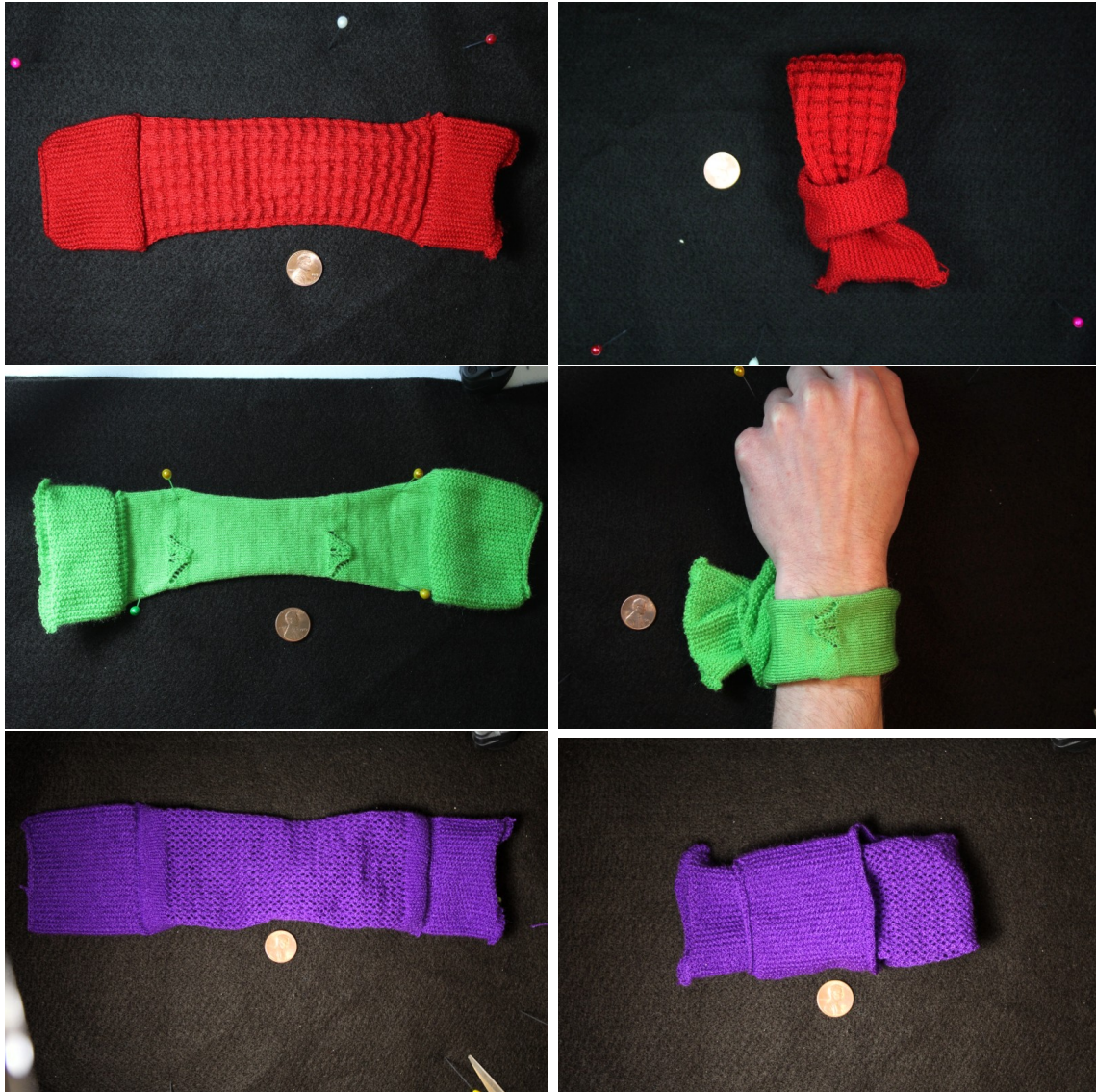
Figure 5-27: The third patterning task required users to transfer an existing pattern onto a provided wristband template. The patterns were either designed by users in a previous step, or selected from our repository of pre-tested designs. The top row shows an expert reference; the middle and bottom rows are from our users.
