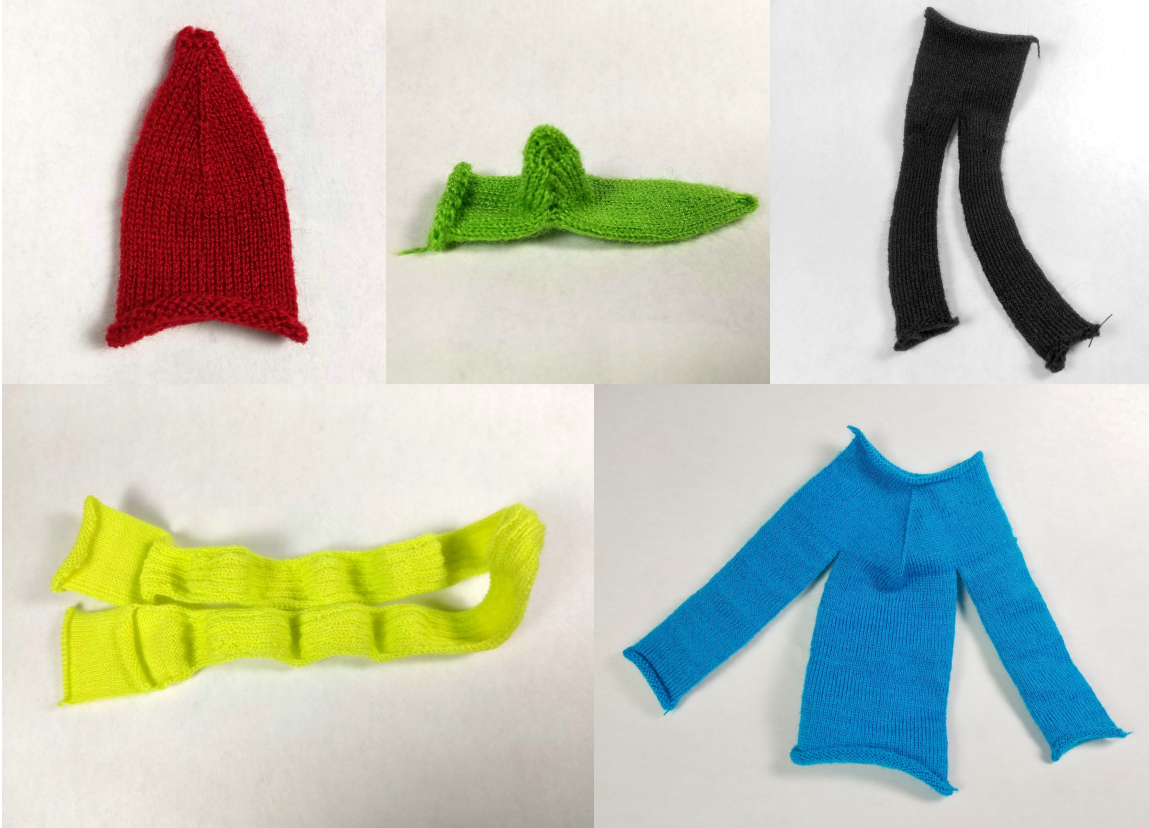
Figure 5-19: The individual garment pieces from the left of Figure 5-17. The scarf uses a single-sided part that would curl on itself by default. Thus we used simple 2 by 2 ribs to keep it flat.
