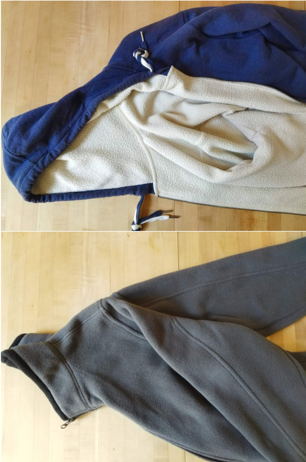
Figure 2-26: Examples of napped fabric used in garments: as an inner layer of a knitted sweatshirt (top) and as an outer layer fleece (bottom).
