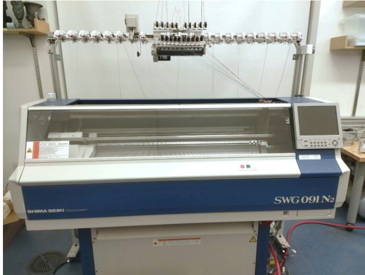
Figure 1-2: The “whole-garment” knitting machine used for the physical fabrication within this thesis – a 15-gauge model SWG091N02 from Shima Seiki [150].
