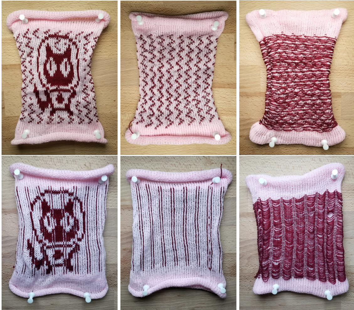
Figure 6-42: Local float patterns typically need accompanying tuck patterns to ensure floats are properly connected to the fabric at regular intervals.
