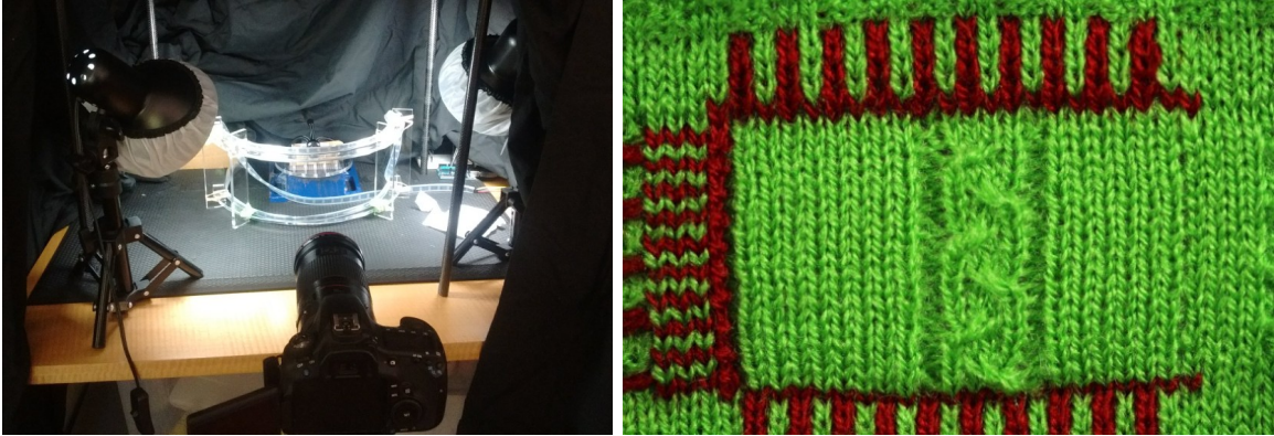
Figure 4-5: Our initial capture setup and a sample pattern illustrating the frame made of intarsia. The pattern tension was controlled with bowel pins inserted at specific holes that were programmed in the fabric.
