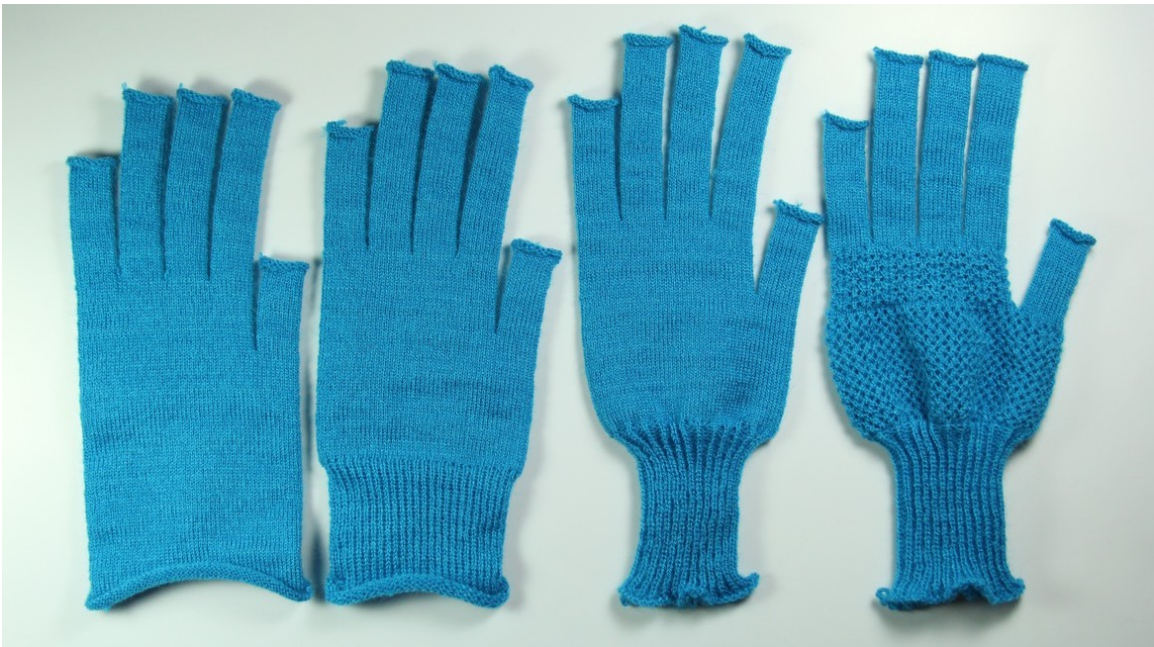
Figure 5-24: Patterning the glove of Figure 5-17 from left to right: base shape, cuff in half gauge, half-gauge cuff with a rib pattern, and final glove with transferred hole pattern on main palm, as well as an additional pattern for the 4-fingers palm.
