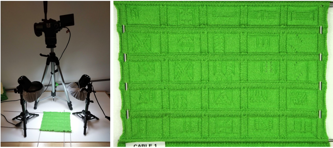
Figure 4-6: Our updated capture setup and a sample of 5 \times 5 knitted patterns with tension controlled by steel rods. In many cases, corner rods were sufficient, whereas more complicated patterns required additional internal rods to reduce the local deformations.
