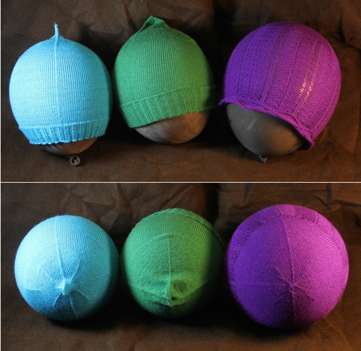
Figure 5-28: A reference beanie on the left and two customized beanies on its right. The rightmost one required a few passes to adjust the lace pattern and its tension.
