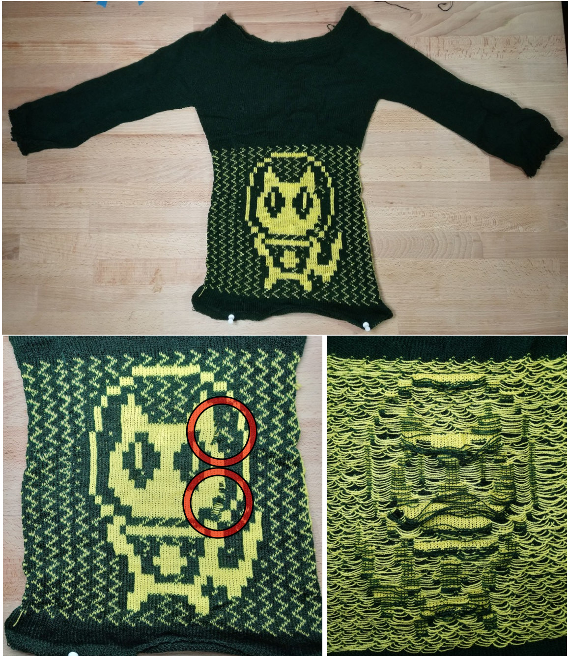
Figure 6-43: A failure example whose main float pattern ends up with too wide floats that lead to failure at their boundaries.
