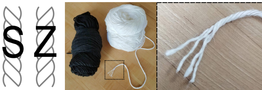
Figure 2-4: Left : the two different twisting directions, often called S and Z twists for the patterns they produces. Right : skeins of yarn and a close-up of their plies.
