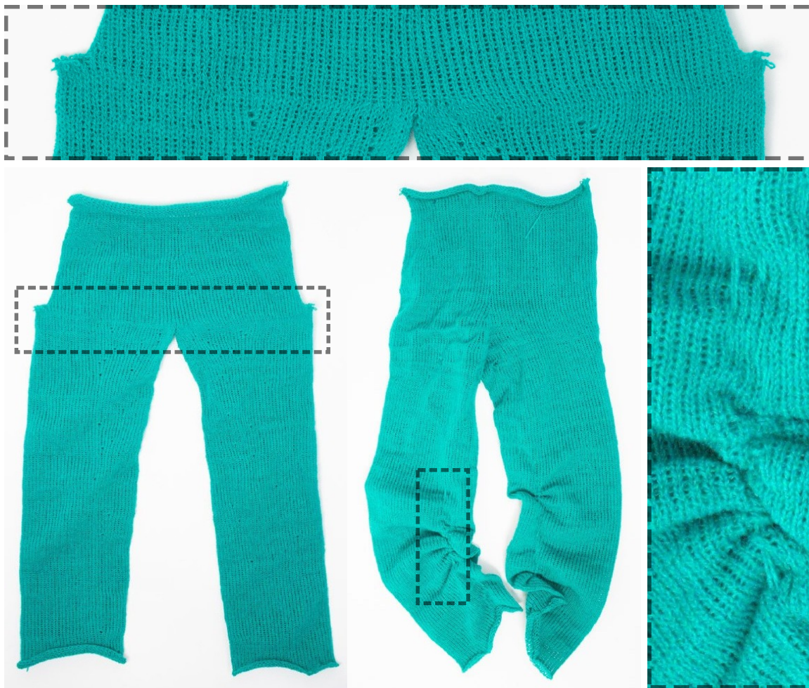
Figure 6-55: Example of knitting failures due to failing needle transfers: the left example failed at large decreases above the crotch due to non-ideal schedule alignments; the right example had catastrophic failures due to overlapping loop transfers during shaping transfers.
