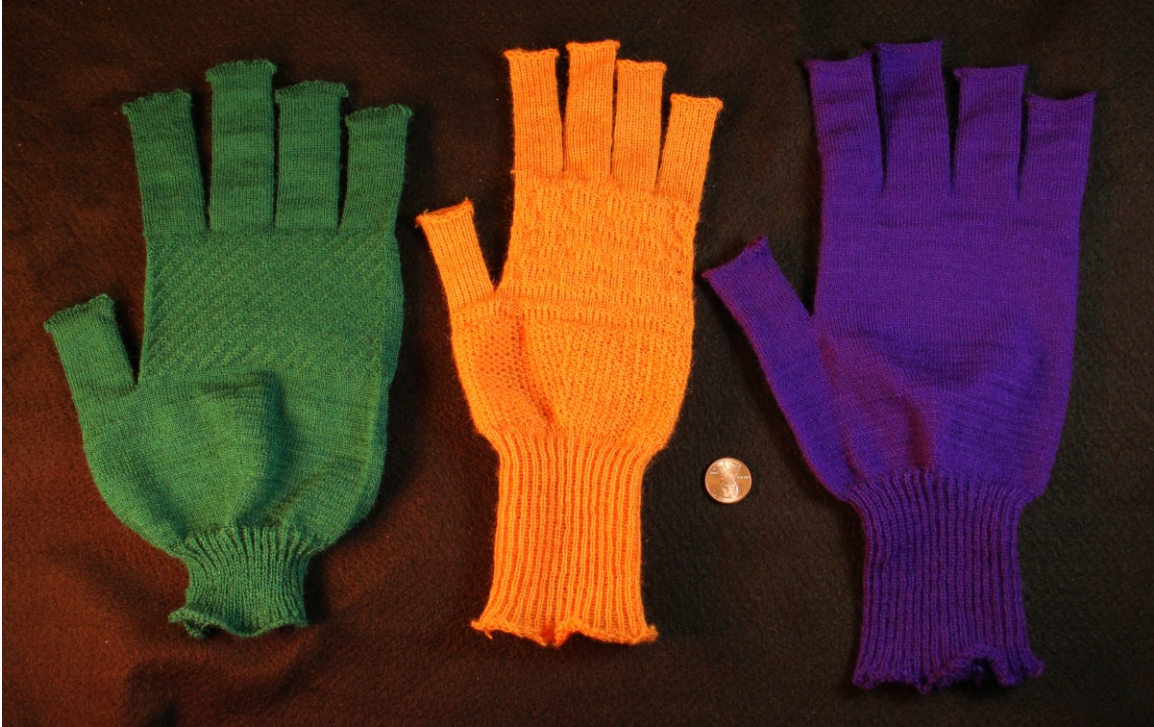
Figure 5-30: Three glove variants. The green one took multiple attempts because of the complicated tension requirements associated with continuous cross patterns.
