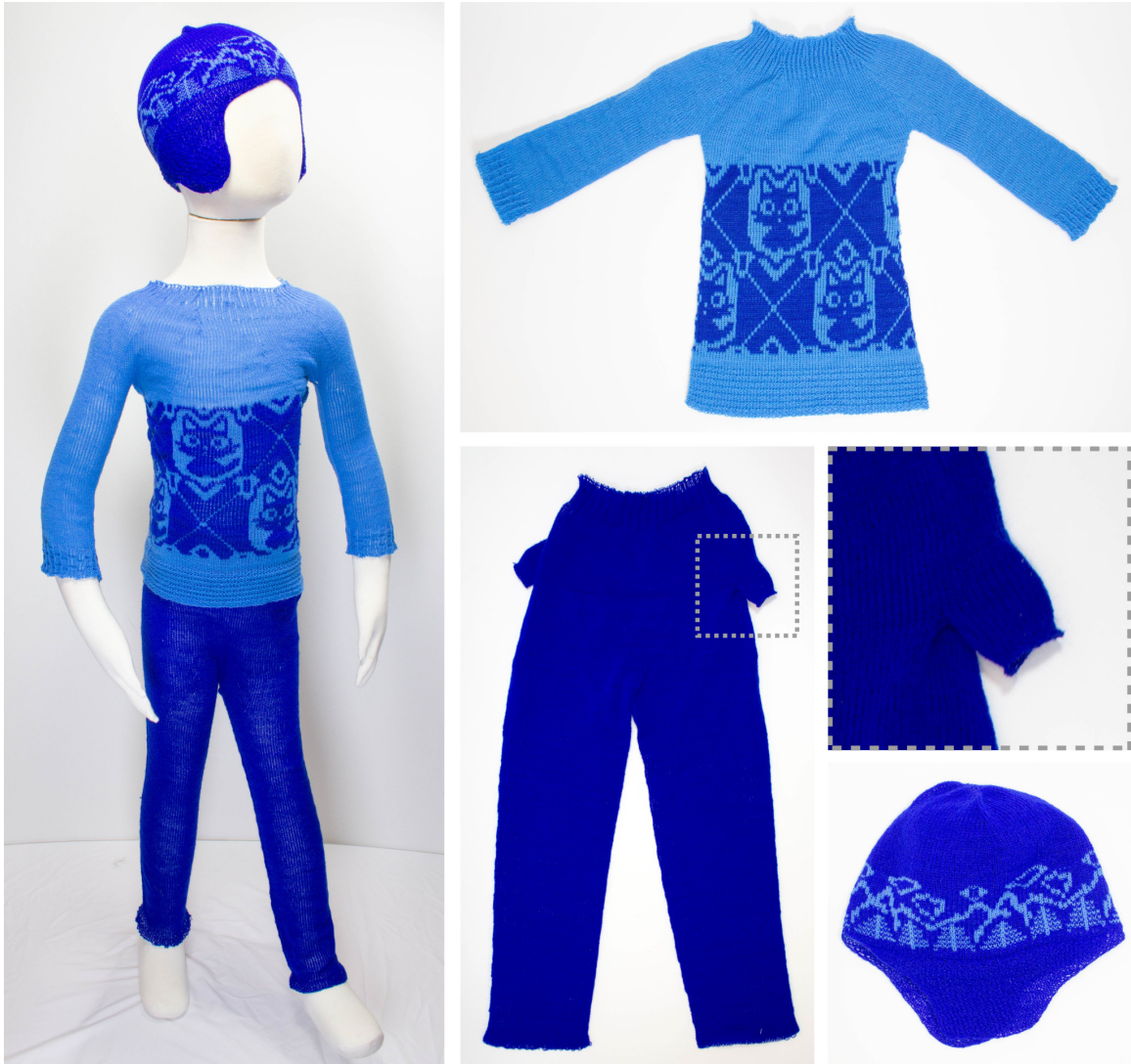
Figure 6-50: Our larger examples on a 4-foot boy mannequin, together with top-down views of the individual garment pieces and a zoom on one of the in-seam pockets of the trousers which are knit as inside-out tubular structures merging with the body.
