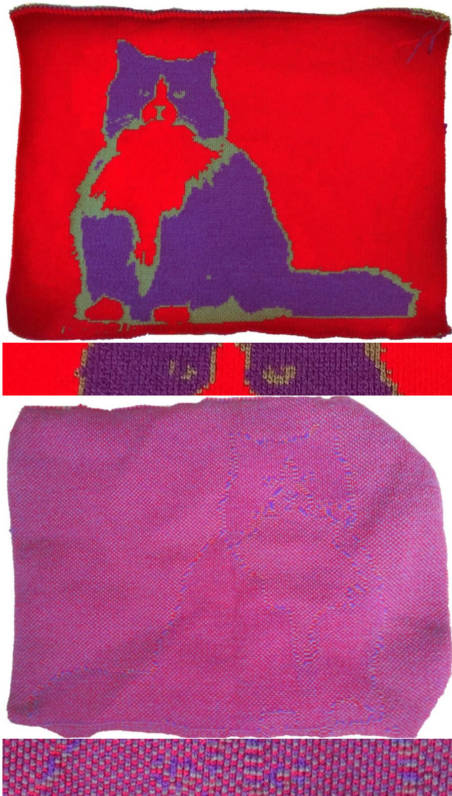
Figure 3-21: Knitted 3-colors jacquard of cat pattern: its front (top) and its back (bottom). The smaller slices are close-ups around the eyes of the cat for both sides.
