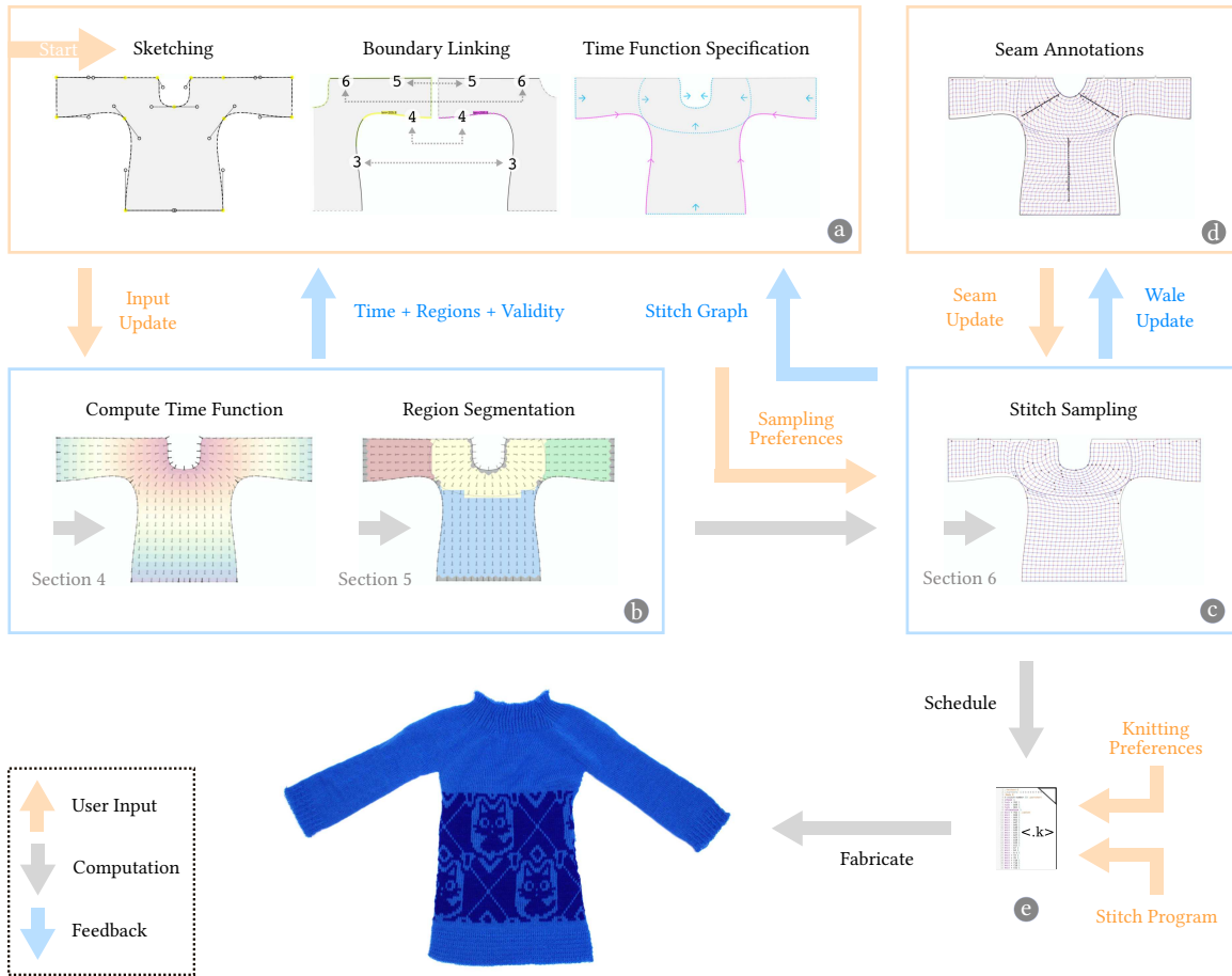
Figure 6-3: Summary of our workflow: (a) the user sketches a garment, links its boundaries and specifies time constraints; (b) the corresponding time function is computed, and its regions segmented; (c) given user sampling preferences (size and course/wale ratios), a stitch graph is sampled; (d) the user can provide additional seam annotations to influence the wale distribution until satisfied; (e) given knitting preferences, a schedule is generated and the physical artifact can then be knitted.
