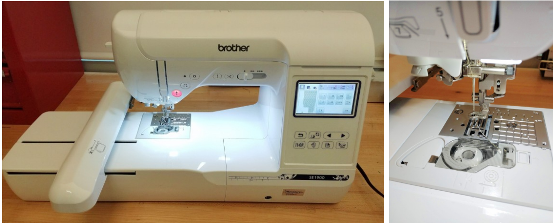
Figure 2-19: A Brother machine for both sewing and embroidery – note the linear gantry (left) – and a close-up looking at the second bobbin that provides the thread below the fabric (right). The main thread comes from above, through the needle.
