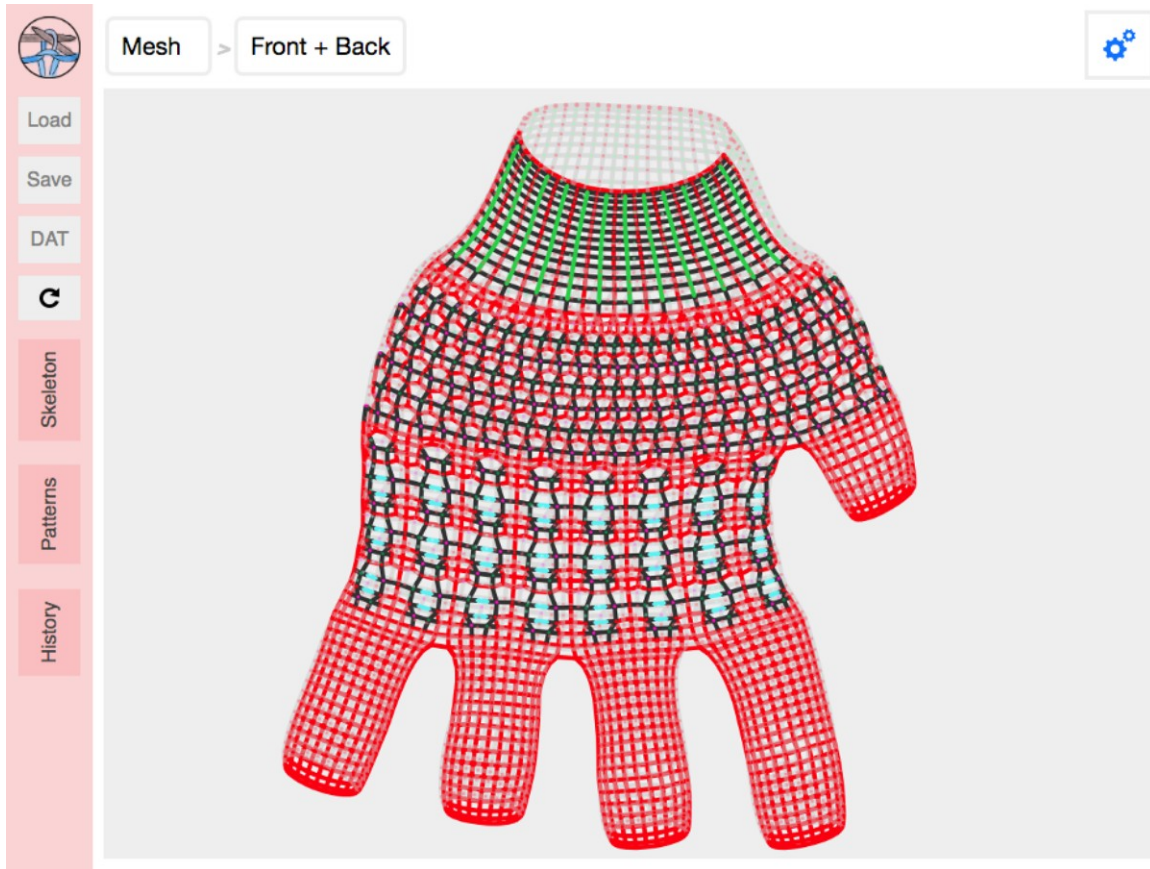
Figure 5-6: Force-layout simulation to preview the impact of the yarn stress forces on the final shape.
