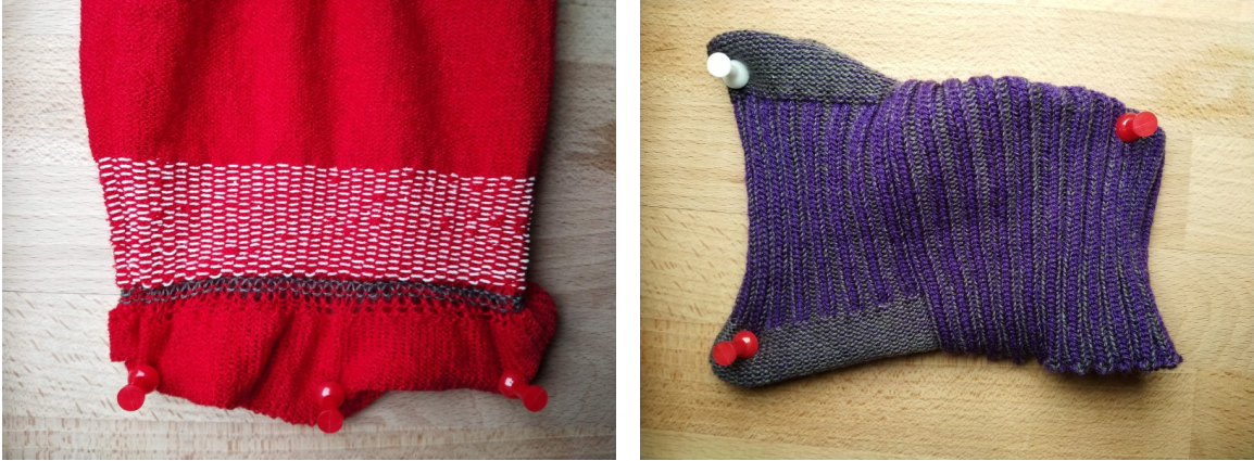
Figure 3-15: Examples using special carrier modes: white inlay yarn (left), gray-blue plated yarn that controls the color side using purls and ribs (right).
