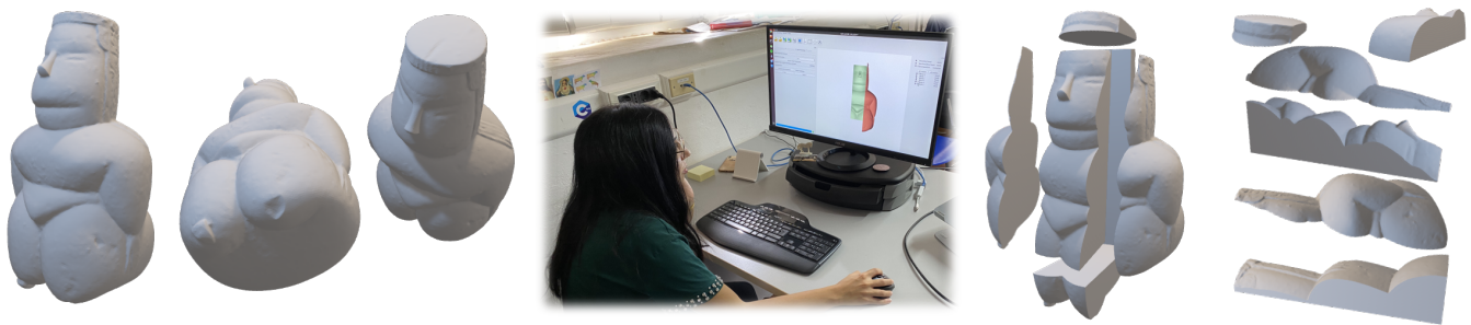
Figure 1: Using Split and Mill the user can interactively look at the digital shape, evaluating which are the best cutting planes to partition it and then generate a subdivision with the guarantee that it is millable with a 3-axis milling machine.
