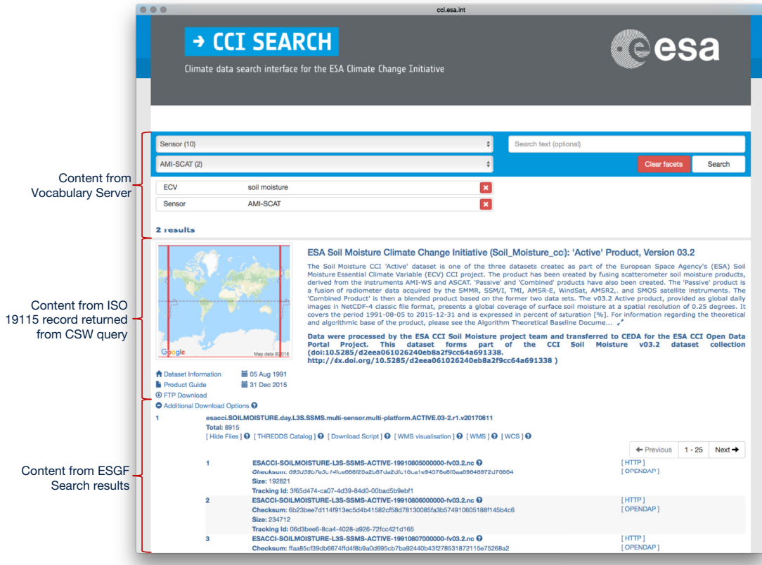
Figure 6: The Web Presence faceted search interface – integrating content from the Vocabulary Server, CSW and ESGF Search services.
