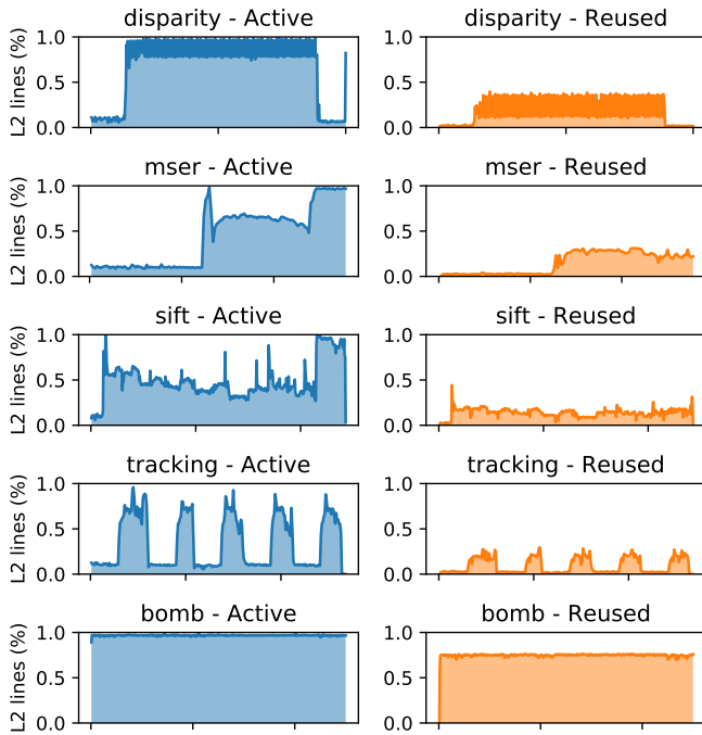
Fig. 12. Active set (left) and reused set (right) analysis of SD-VBS and BOMB benchmarks.
