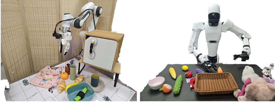
Fig. 7: Evaluation Setup. The evaluation uses two robot platforms: the Franka Panda (left), for 6 short-horizon tasks; and the AstriBot-S1 (right), for 2 long-horizon tasks.
