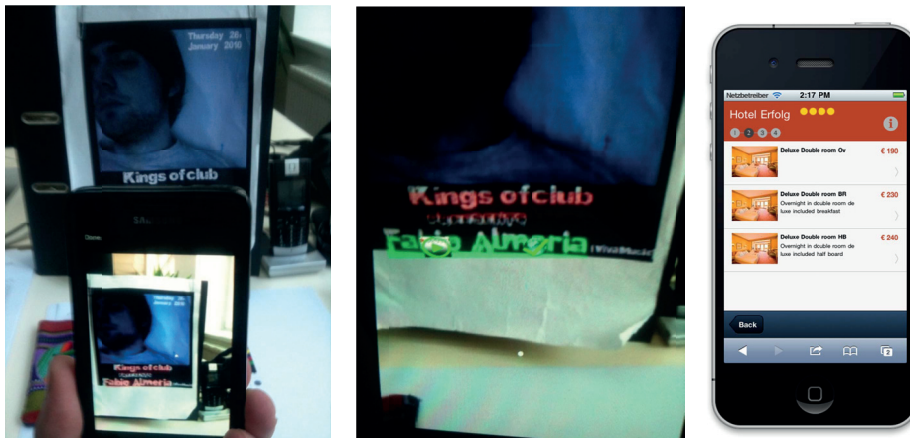
Fig. 4. SmartReality view in the client. Left: poster is recognized and the regions with content are indicated. Middle: on pressing a content region, the available content items are shown. Here the artist Fabio Almeria is associated with an audio stream from play.fm and a web link to booking a hotel room for after his next concert from Seekda. Right: following the web link the user is at a hotel room booking screen (date and location is not input, as it is known from the event’s description)
